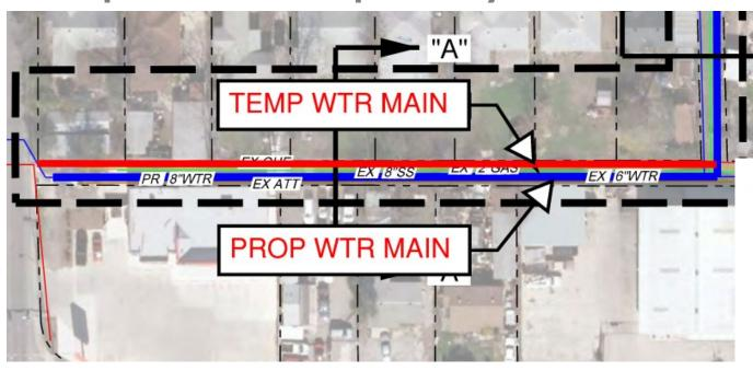
There will be a temporary water main installed in the \_ \_ \_ \_ alley off of Culebra. The existing water mains located EXIST/PROP MB - along the alleys off of Culebra and Tulane will be removed and replaced in place.
